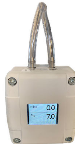
Monitoring filter condition (DDMU)
